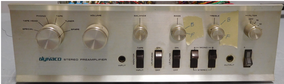
Figure 2-Mark the fully clockwise positions of the front and back tone control knobs
