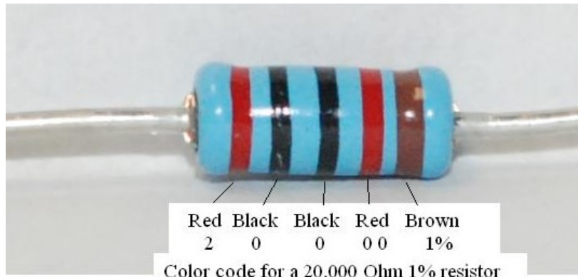
Figure 11-demonstrating the resistor color code
