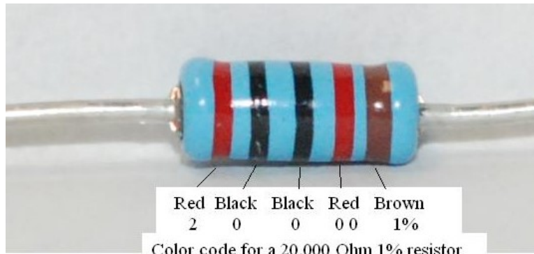
Figure 13-demonstrating the resistor color code
