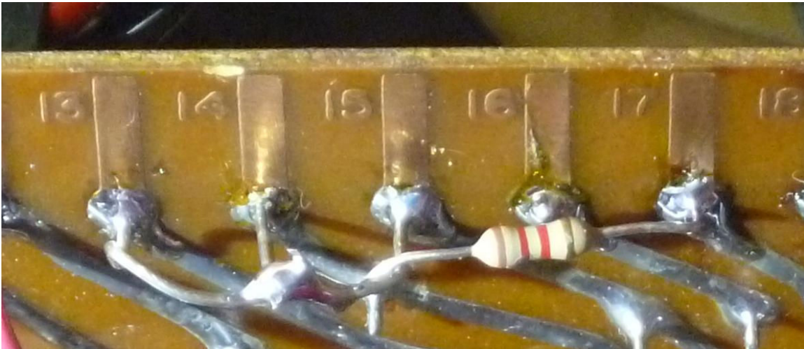
Figure 1-modification connects eyelets 13, 14, and 15 together. The combined node connects to eyelet 17 via a 1200 Ohm resistor (only one channel shown here, both channels must be converted).
