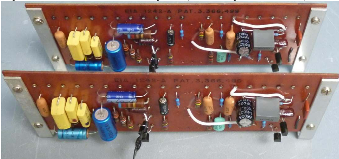
Figure 7-Both PCBs reassembled onto U brackets, ready for installation (DRD4 kit installed also)
