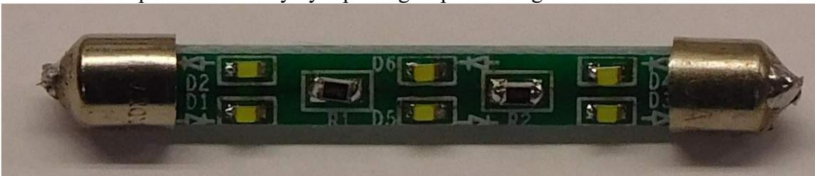
Figure 9-Complete LED based cartridge lamp replacement
