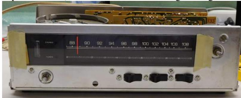
**Figure 3-Nuts holding front panel were removed, and front panel has been removed**
