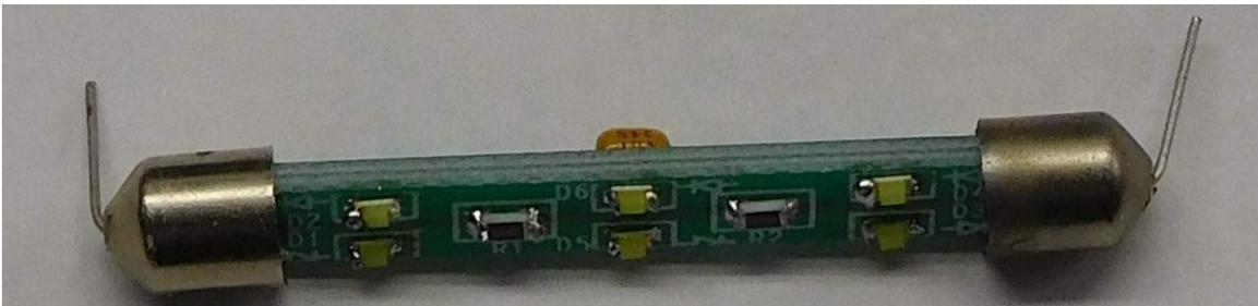
Figure 8-Replace the end caps and bend the wires
