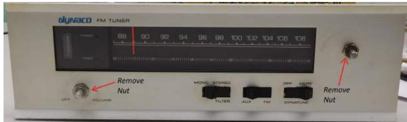
**Figure 2-Remove two nuts, then remove front panel**
