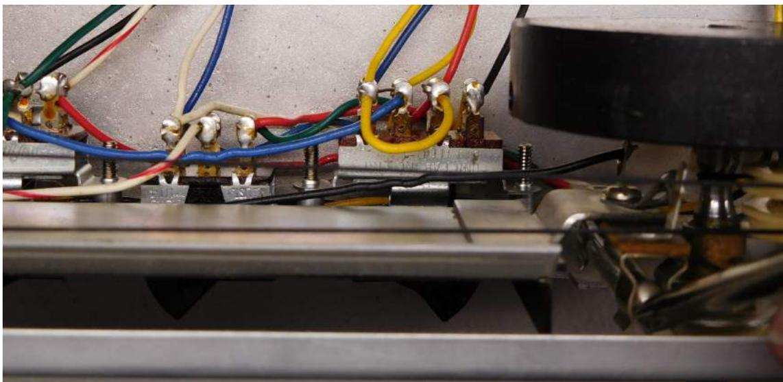
**Figure 4-Push down, then finagle back, to remove the cartridge lamps**
