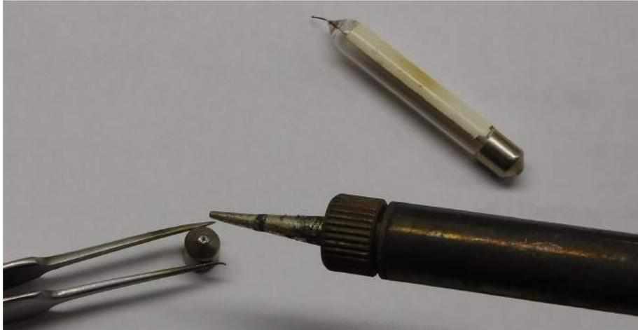
**Figure 5-Harvesting and de-soldering the end caps**
