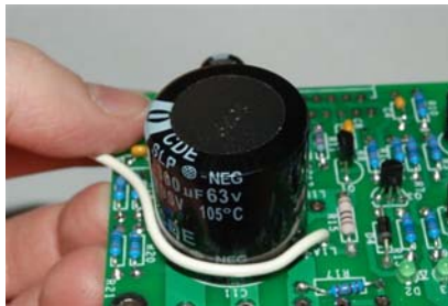
Figure 12-Starting to wind the output inductor
