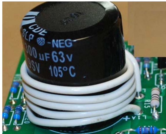
Figure 13-finishing step for the output inductor
