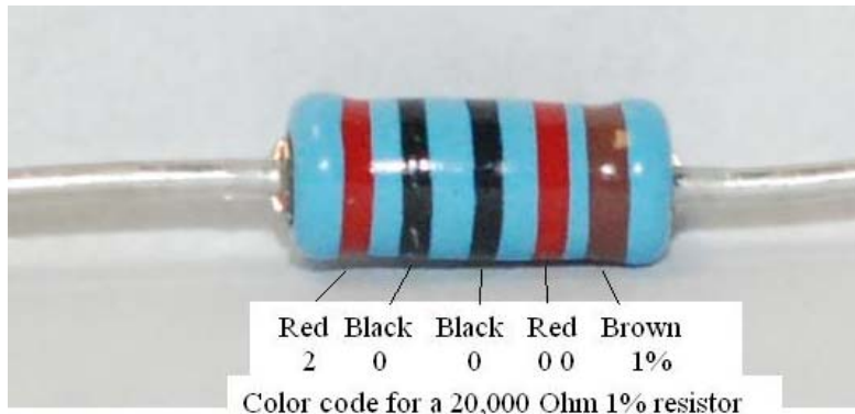
Figure 22-demonstrating the resistor color code
