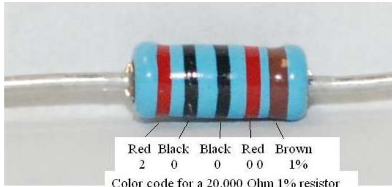
Figure 22-demonstrating the resistor color code
