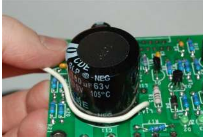
Figure 12-Starting to wind the output inductor
