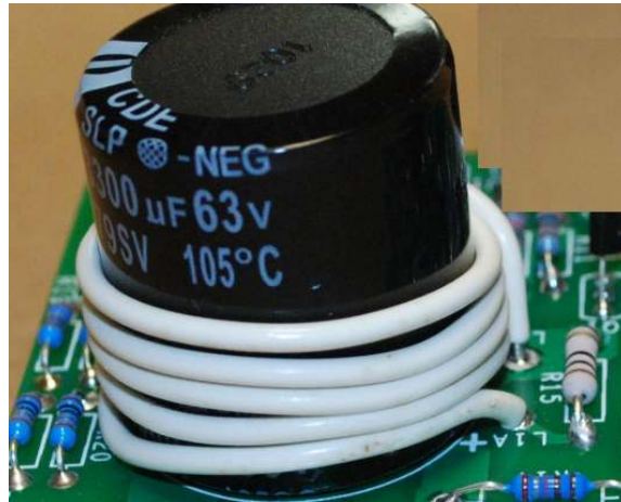
Figure 13-finishing step for the output inductor
