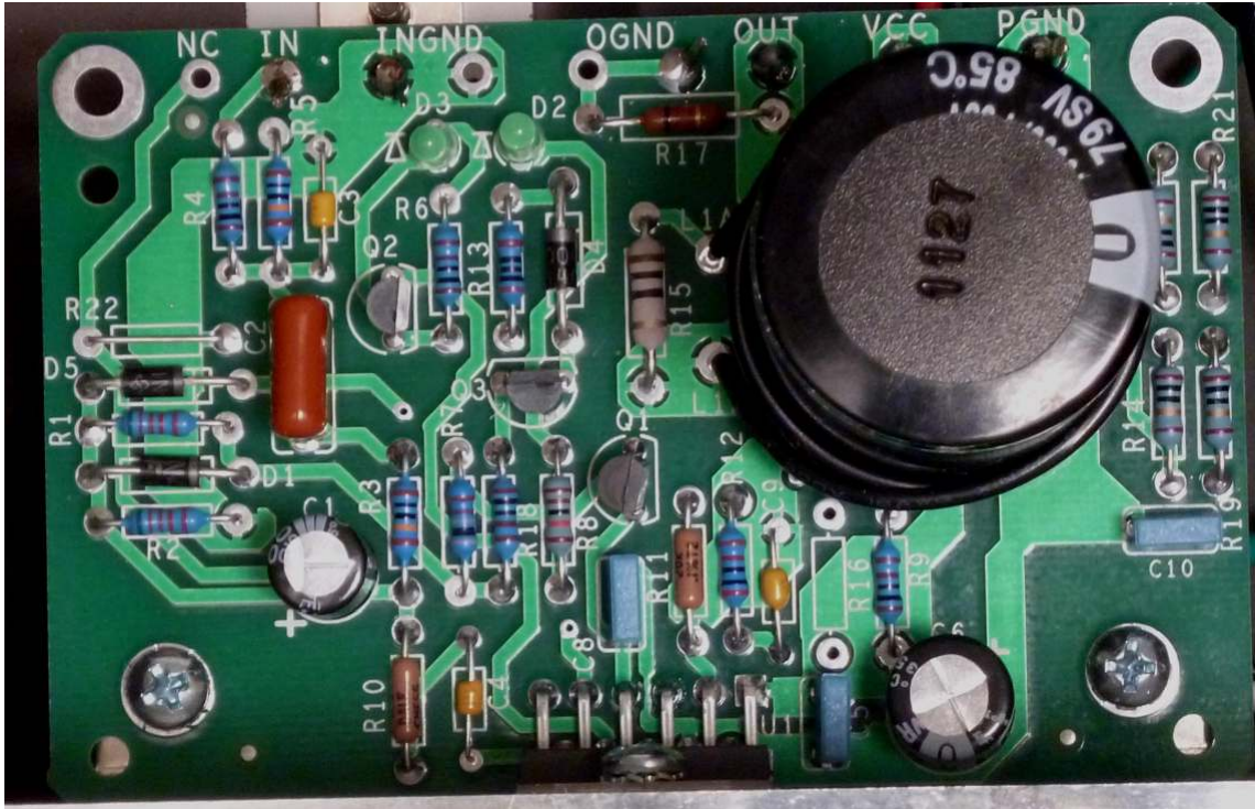
Figure 8-Closeup of Completed Amplifier board (your big cap may look a bit different)
