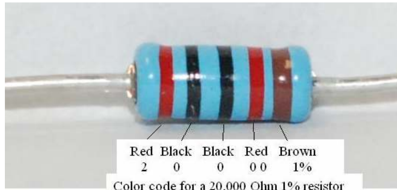
Figure 24-demonstrating the resistor color code
