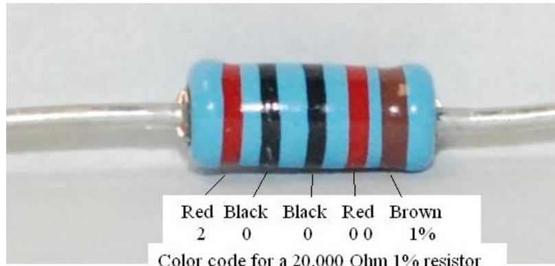
Figure 14-demonstrating the resistor color code
