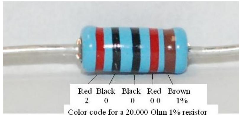
Figure 14-demonstrating the resistor color code
