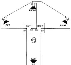
Best results occur when all speakers have identical efficiency, impedance and sonic characteristics, as separate level controls are not feasible. The front speakers should be matched in any case. Dynaco speakers, with very uniform impedance characteristics, are ideal, and permit the A-50 to be used with the A-25 with outstanding results.
