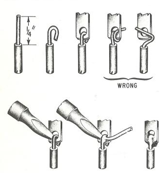
When soldering a lead to an eyelet on the circuit board, the Stereo 120 makes it easy to apply the iron to one side of the board while the tinned wire end is pressed into the solder-filled eyelet from the opposite side. When the eyelet is heated, the wire enters easily, but be careful that you do not push the wire all the way into the eyelet up to the insulation. If you do, you will not be
