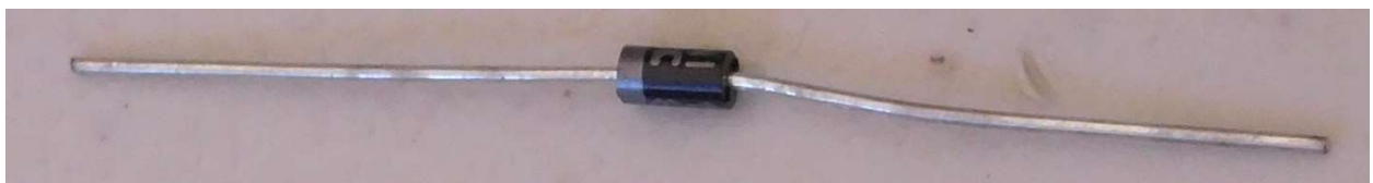
Figure 13-Diode. Note the band on the left side!
