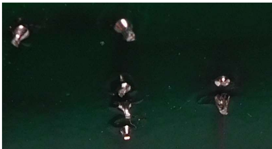
Figure 10-clipped leads protrude past the solder volcano
