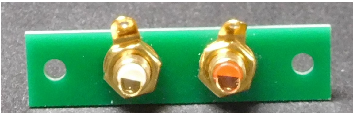
Figure 4-Building the new RCA jack assembly, back view
