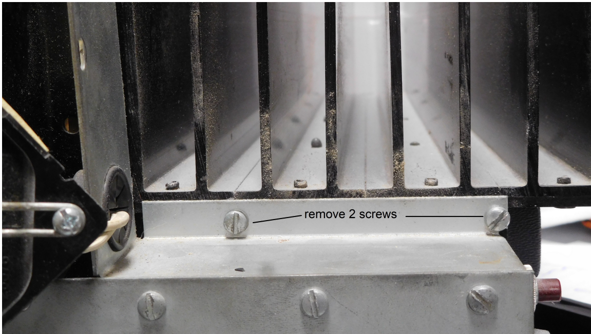
Figure 6-Remove two screws from the side, behind the fan Remove two side screws, on the non-fan side of the chassis.
