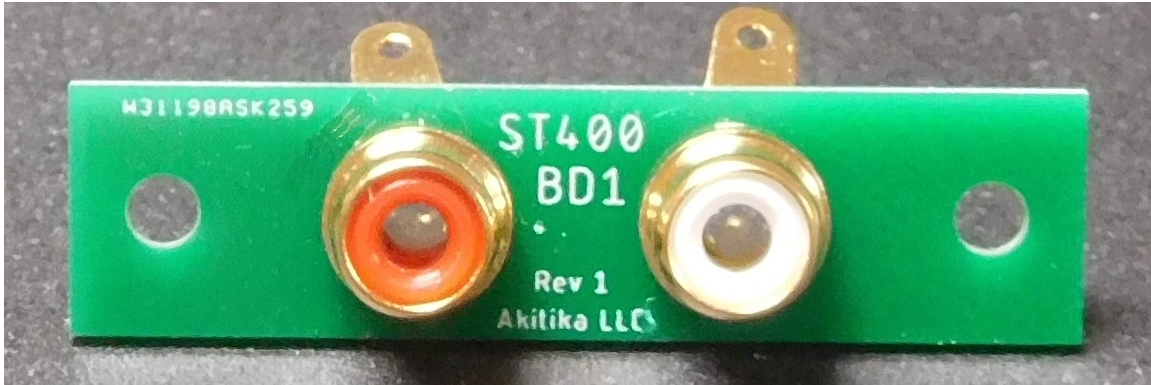
Figure 3-Building the new RCA jack assembly, front view
