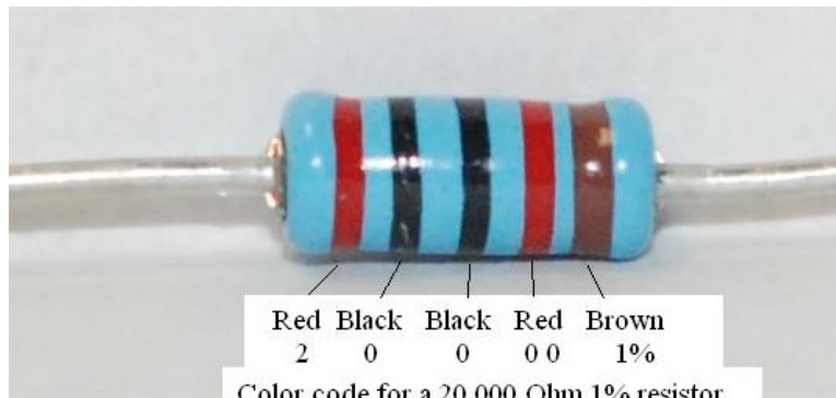
Figure 21-demonstrating the resistor color code
