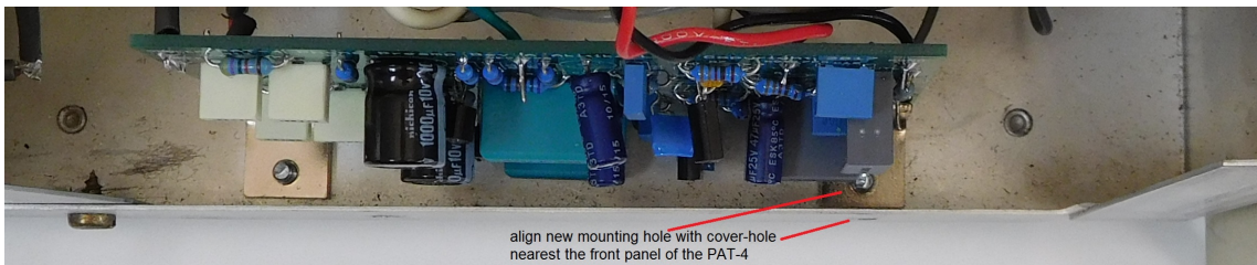
Figure 5-Locating the mounting holes
