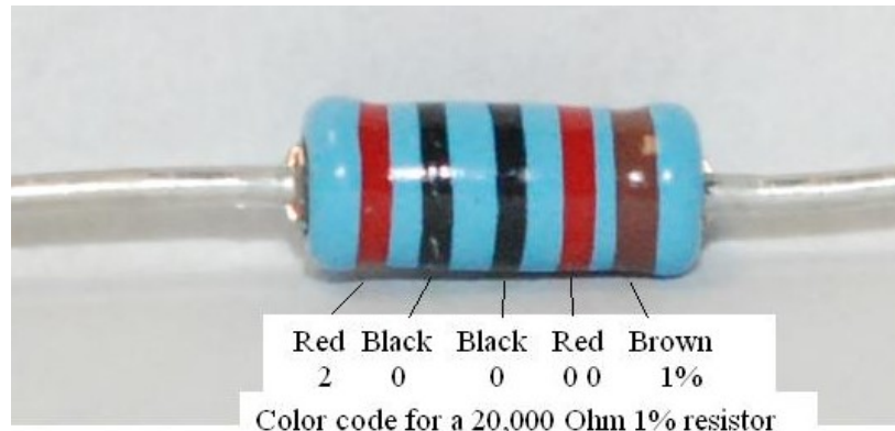
Figure 7-demonstrating the resistor color code
