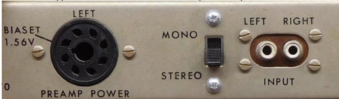
Figure 3-Installed new stereo/mono switch
