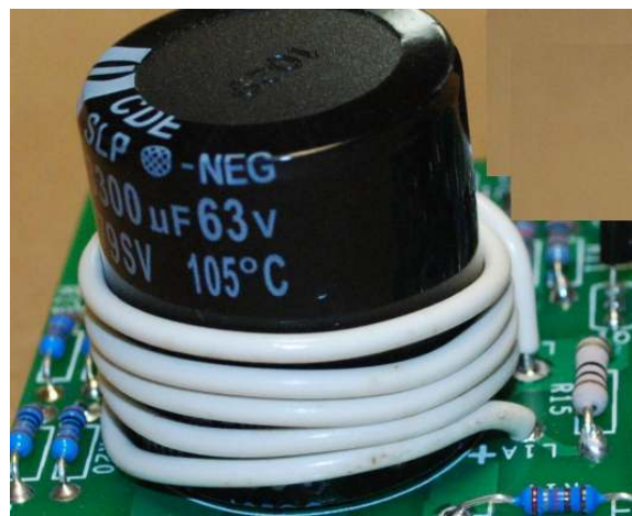
Figure 11-finishing step for the output inductor
