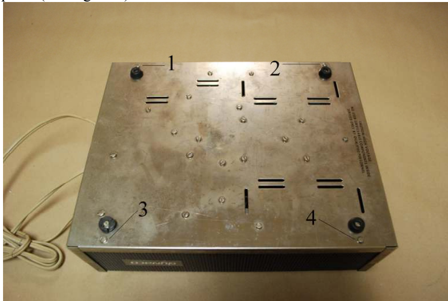
Figure 1-Location of the four screws that hold the cover to the base
