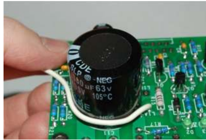
Figure 10-Starting to wind the output inductor
