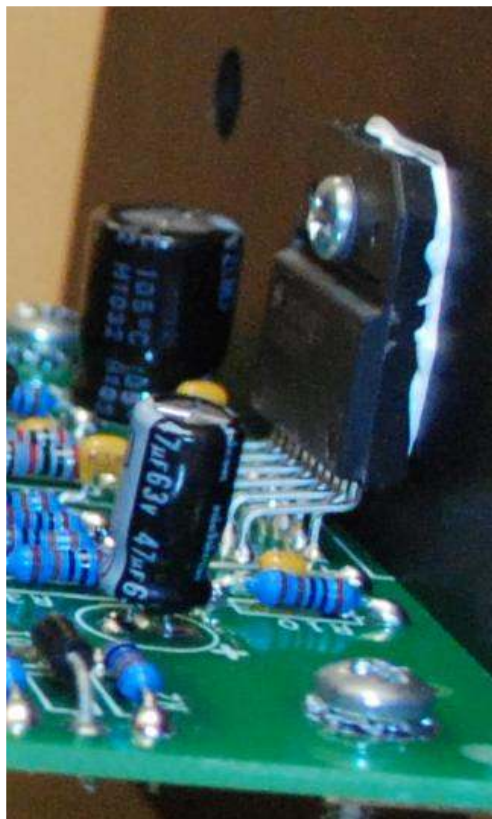
Figure 15-The LM3886 sits up off the board to avoid shorts between the front and back rows of pins. The body should be at right angles to the circuit board
