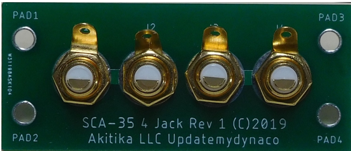
Figure 2-Jack installation, (left channel, white insulator jacks shown)
