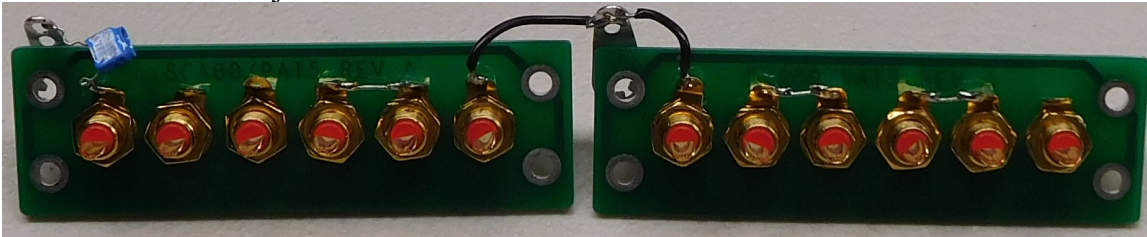
Figure 3-Right Channel Jacks with grounds and 0.01 uF cap
