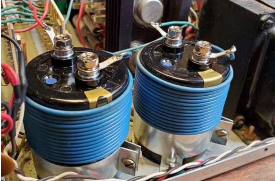
Figure 12-Installing C7X2C into a stock SCA80(Q)
