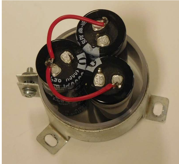
Figure 6-Connecting the positive terminals together
