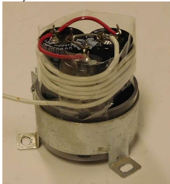
Figure 9-Adding tape to hold the windings (optional)
