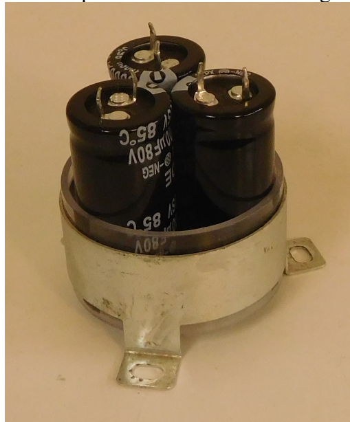
Figure 5-3 capacitors take the space of one 2” diameter capacitor
