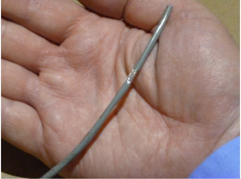
Pull the insulating jacket off, exposing the cable, showing the foil shield, the drain wire,
