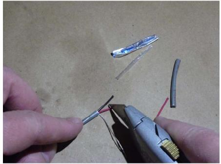
Remove a bit of insulation using diagonal cutters, starting from the knife score-line.
