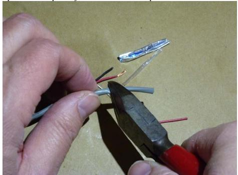
Tin the drain wire and the red wire. You might also want to strip and tin the black wire, depending upon your application. Slide the insulator onto the drain wire. The end is now prepared for installation.
