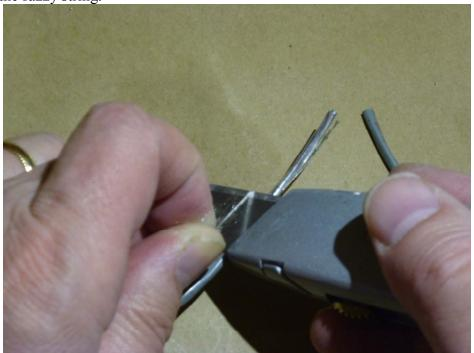
Separate and twist the drain wire.
