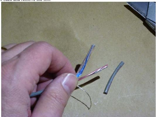
Remove the plastic wrap from the red and black wires.
