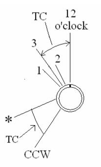
Figure 3 - \* marks the new position for the CCW extreme of the pot's travel
