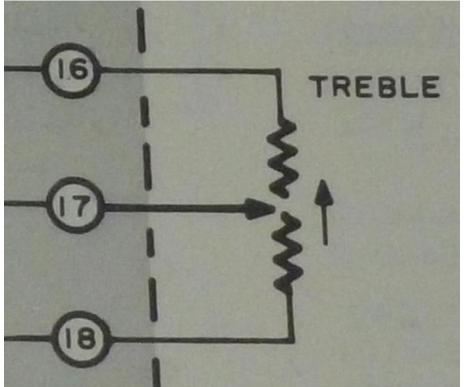
Figure 1 – close-up of the drawing of the treble pot in the PAT-4 schematic clearly shows the break in the center of the resistive element
