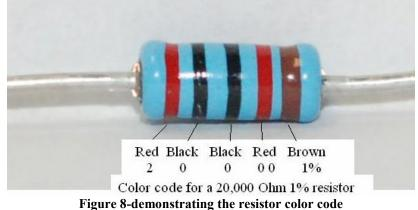
Here's an extreme close-up of a 1/4 W metal film 20K (20,000) Ohm resistor, designated by the standard resistor color code.
