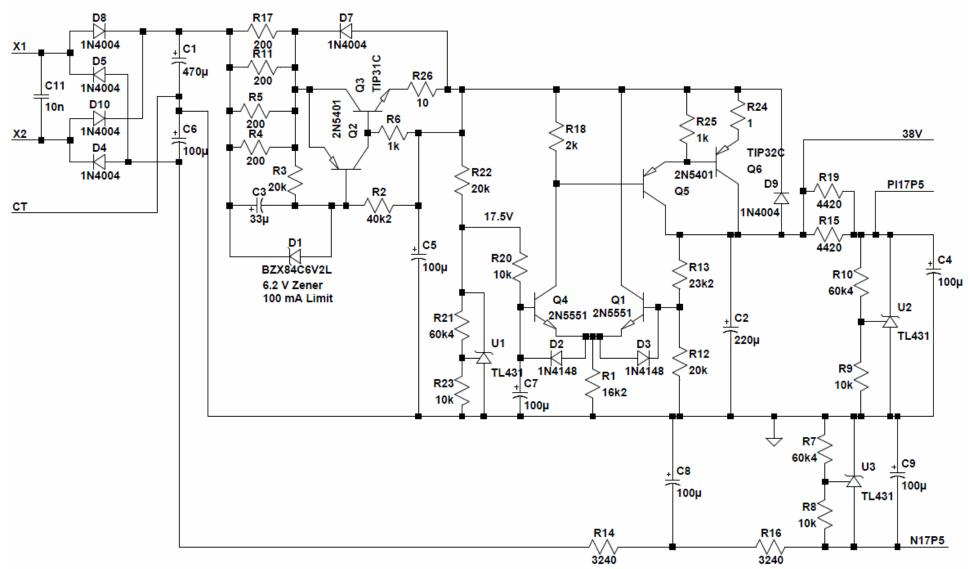
Figure 7-Schematic of the PAT-4 Electronically Regulated Power Supply. Note that Q6 has a heatsink
