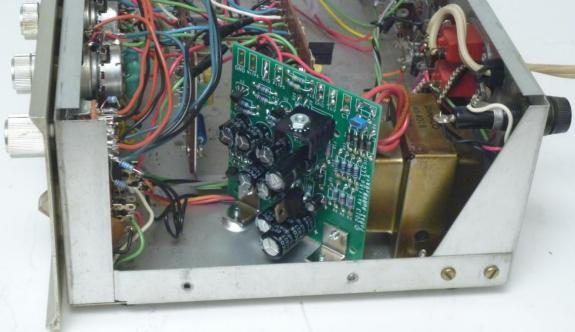
**Figure 6-New Power Supply Installed in PAT-4 (this PAT-4 has tone control defeat switch)** If the voltages check out in the previous step, then:
