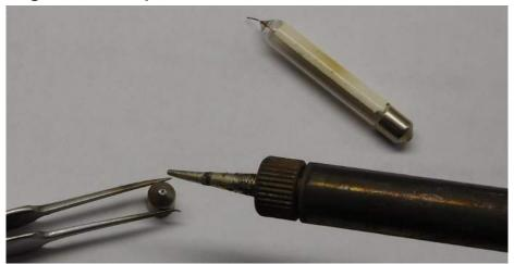
Figure 5-Harvesting and de-soldering the end caps
