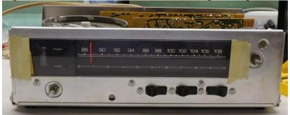
Figure 3-Nuts holding front panel were removed, and front panel has been removed
