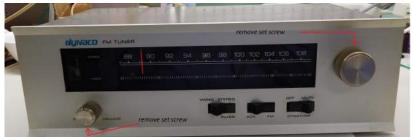
Figure 1-Loosen the set screws and remove the knobs
