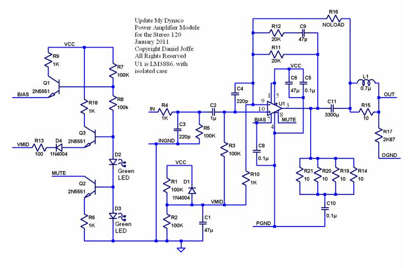
Figure 22-Schematic of amplifier module
