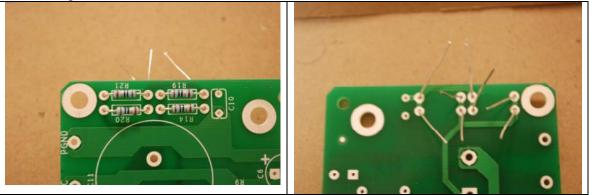
Figure 10-The first four resistors are installed with leads bent on the back side, but not yet soldered.
