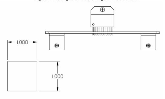
Figure 16-Template for checking mounting height of LM3886
