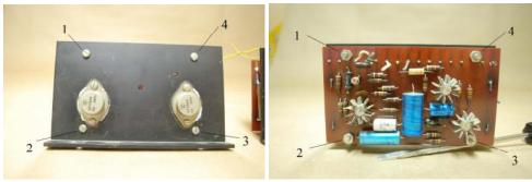
Figure 5- Separating heat sinks and circuit boards
