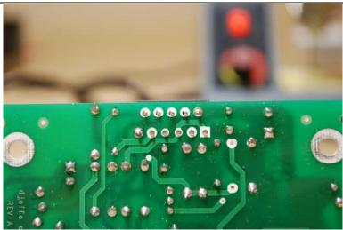
Figure 17-LM3886 installation step three, just the corner pins are soldered
