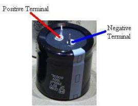
Figure 7-Identifying the positive and negative terminals
