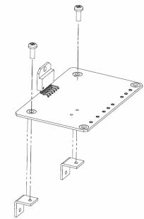
Figure 15-Showing method of attaching brackets to the PCB
