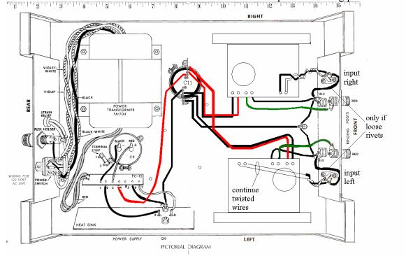
Figure 21-completed wiring
