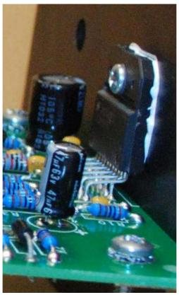
Figure 18-The LM3886 sits up off the board to avoid shorts between the front and back rows of pins. The body should be at right angles to the circuit board
