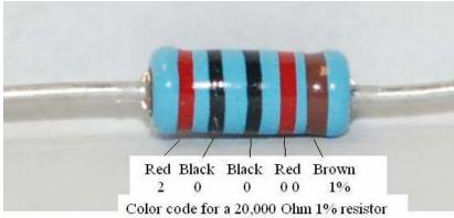
Figure 23-demonstrating the resistor color code
