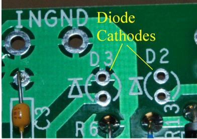
Figure 12-showing LED cathode orientation
