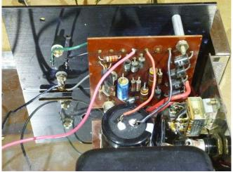
Figure 8 - showing the new C9 installed.
