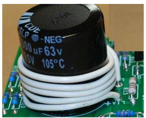
Figure 14-finishing step for the output inductor
