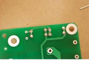
Figure 11-leads soldered and clipped
