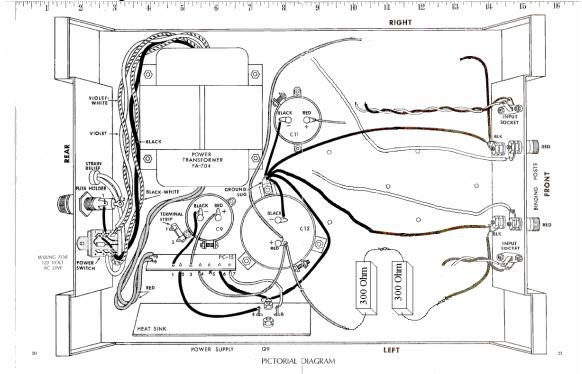
Figure 6-Connecting a test load to the power supply
