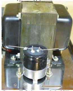
Figure 9 - crimp and solder "antenna-like" wires to terminals of C11 to facilitate the connection of the power supply and amplifier wires
