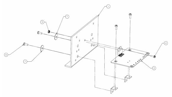
Figure 19-Mounting assembled PCB to heat sink
