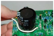
Figure 13-Starting to wind the output inductor
