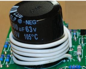
Figure 10-finishing step for the output inductor
