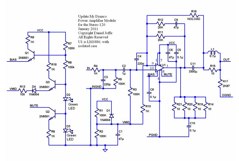
Figure 20-Schematic of amplifier module
