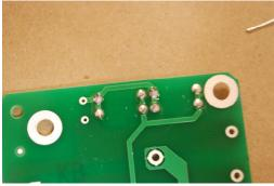
Figure 7-leads soldered and clipped
