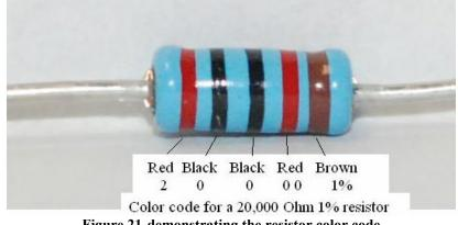
Figure 21-demonstrating the resistor color code
