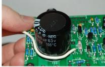
Figure 9-Starting to wind the output inductor
