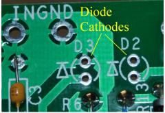
Figure 8-showing LED cathode orientation
