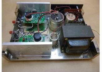
Figure 16-Showing the Final Wiring (shown with isolated, rather than original input jacks)
