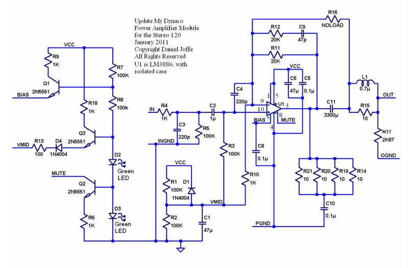
Figure 19-Schematic of amplifier module
