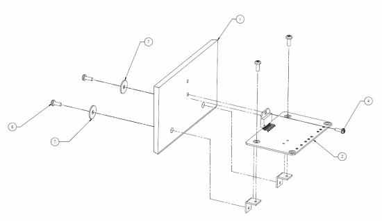
Figure 14-Assembling the circuit board to the heat sink
