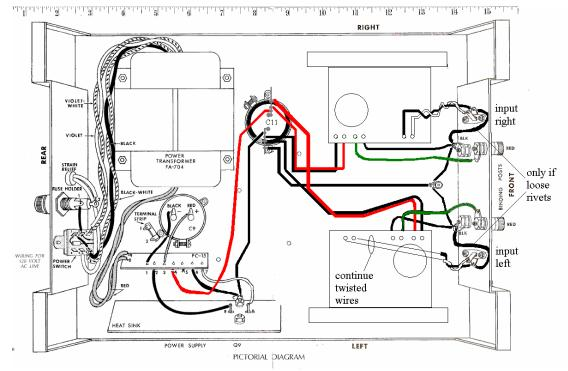
Figure 18-completed wiring
