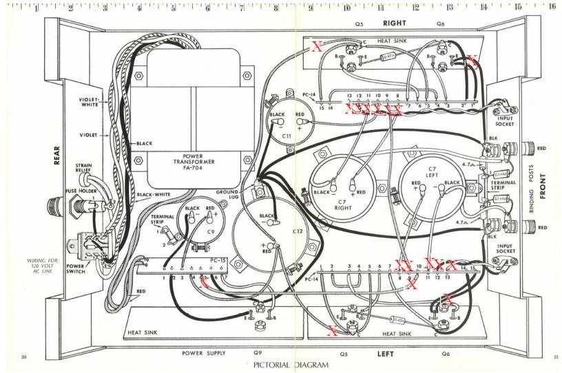
Figure 2-Location diagram for cutting wires
