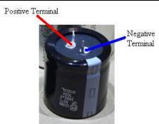
Figure 6-Identifying the positive and negative terminals
