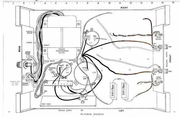
Figure 5-Connecting a test load to the power supply
