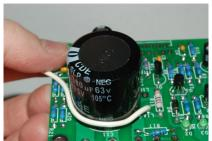
Figure 12-Starting to wind the output inductor
