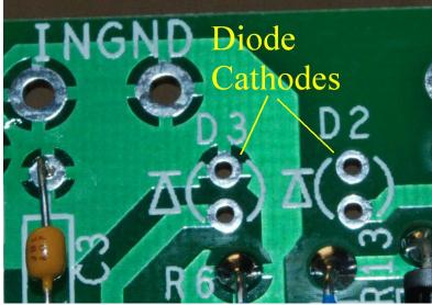
Figure 11-showing LED cathode orientation
