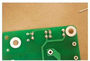
Figure 10-leads soldered and clipped
