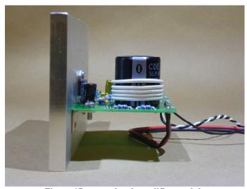
Figure 17-a completed amplifier module
