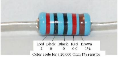
Figure 20-demonstrating the resistor color code
