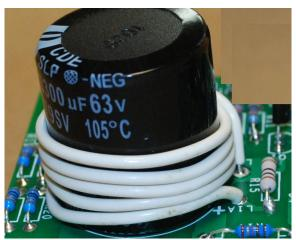
Figure 13-finishing step for the output inductor
