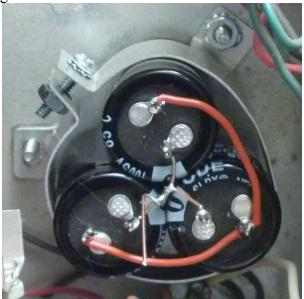
Figure 4-Soldering the ground positive harnesses on the new C9 dynamite capacitor arrangement
