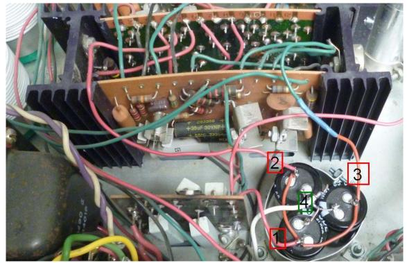
Figure 6-Reconnecting the wires to the new C9
