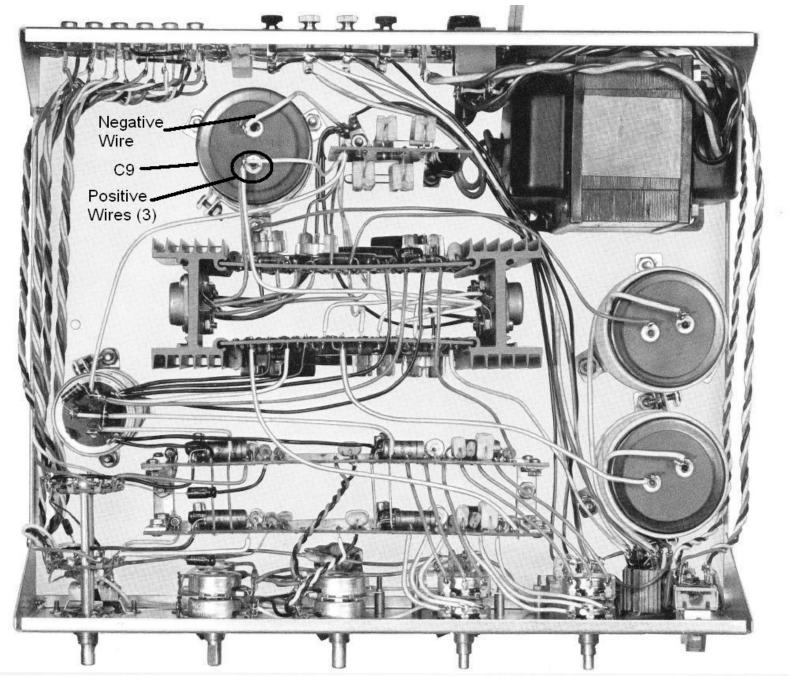
Figure 7-Stock amplifier layout (before C9 replacement)
