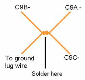
**Figure 3-Ground Harness Configuration**
