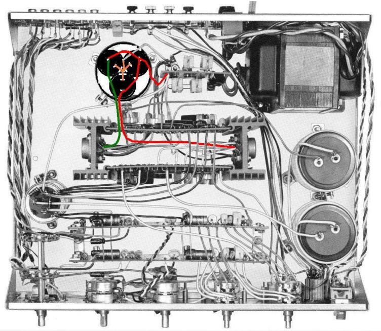
Figure 8-Stock Amplifier with Dynamite Capacitor Configuration Installed
