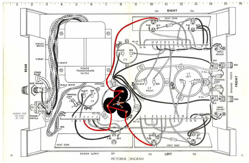
Figure 6-Stock Amplifier with Dynamite Capacitor Configuration Installed
