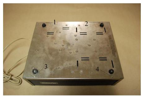
Figure 1-Location of the four screws that hold the cover to the base If the voltage on C12 was within tolerance, then:
