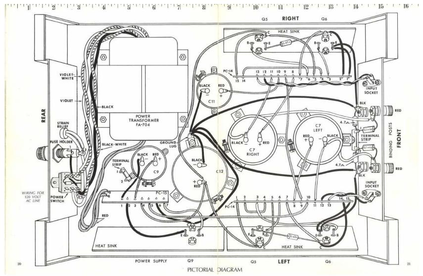
Figure 5-Stock amplifier layout (before C12 replacement)
