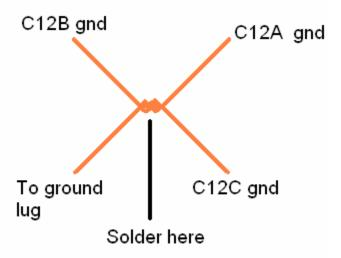
**Figure 4-Ground Harness Configuration**
