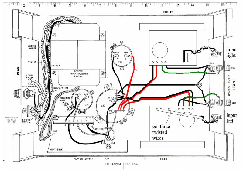
Figure 7-Dynaco PC-15 Power Supply and Updatemydynaco amplifier modules, before changing C12
