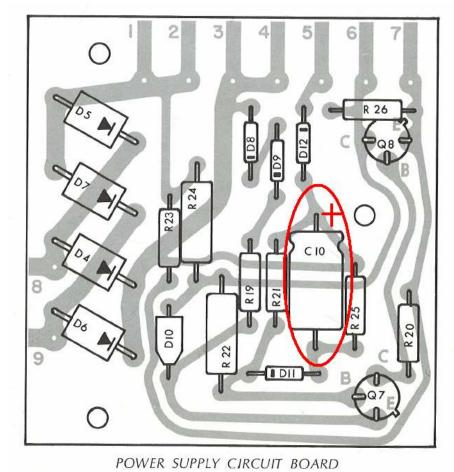
Figure 2-Dynaco PC-15 Power supply board highlighting C10 location and polarity
