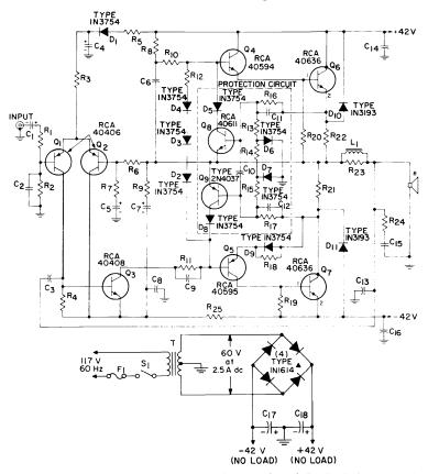
NOTES: (1) Output transistors  $Q_0$  and  $Q_7$  and diodes  $D_2$  through  $D_4$  should be mounted on a common heat sink (Wakefield Type NC-403K or equiv.). Diodes should be attached to under side of heat sink by use of small metal cable clamps. (2) Transistors  $Q_1$  and  $Q_2$  should be matched for base-to-emitter voltage within 0.04 volt and should be selected for a beta between 100 and 300 at 1 milliampere and 5 volts.
