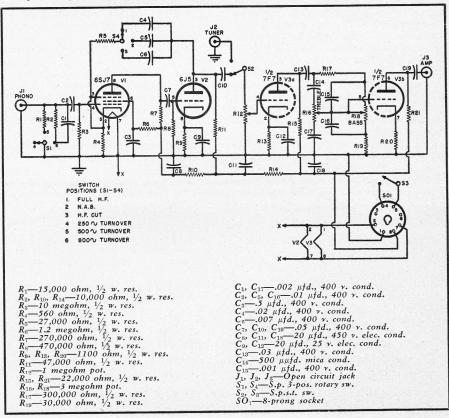
Fig. 3. Suggested preamplifier incorporating tone controls and equalizing networks.
