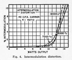
the normal plate supply voltage of 425 volts, about 15% more output or 11.5 watts can be expected for the same amount of intermodulation distortion.
