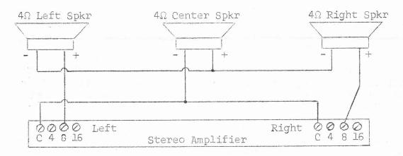
Note: 4 ohm speakers shown connect to 8 ohm amplifier taps. 8 and 16 ohm speakers connect to 16 ohm amplifier taps.
