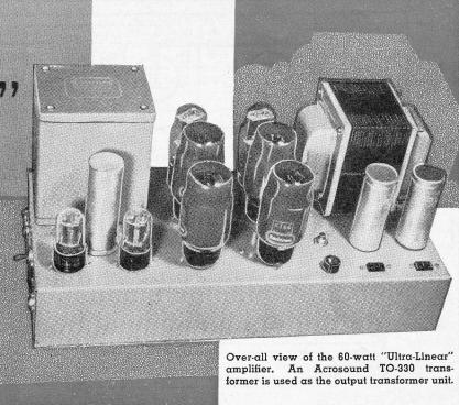
Construction details on a commercially-designed, high-power amplifier for the serious audiophile. It uses four KT66's.
